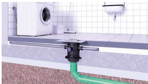
Installation with waterproofing against groundwater
