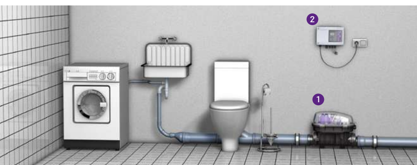
1 Backwater pumping station 2 Control unit
