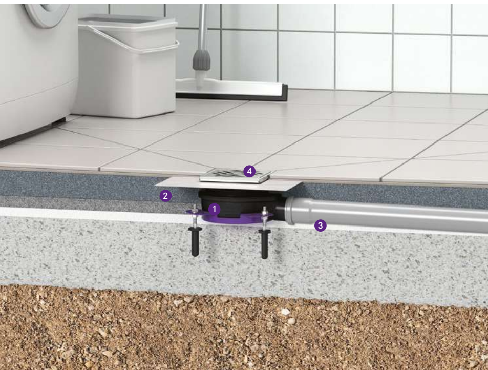
1 Drain 2 Waterproofing membrane 3 Drain pipe 4 Cover
