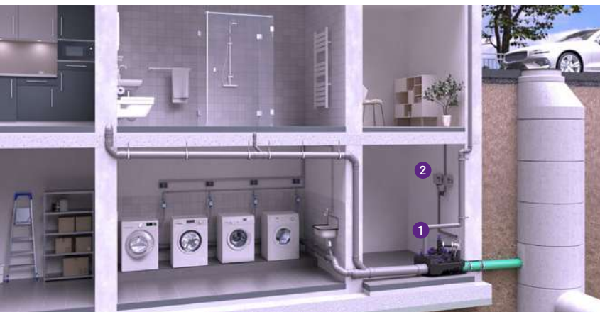
1 Hybrid lifting station 2 Control unit
