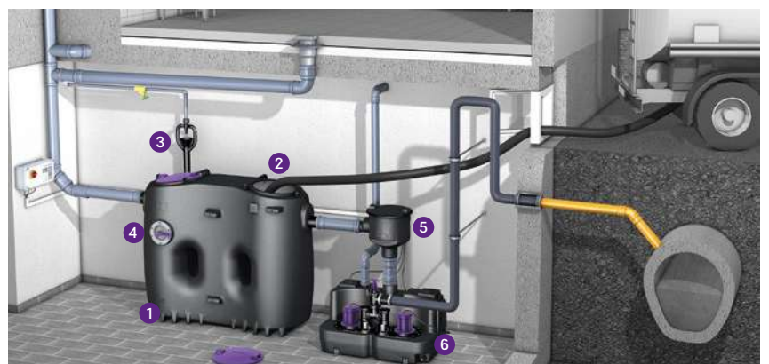
➊ Grease separator EasyClean free Basic Standard ➋ Emptying takes place by opening the separator ➌ Refill inlet ➍ Inspection window ➎ Sampling chamber ➏ Lifting station
