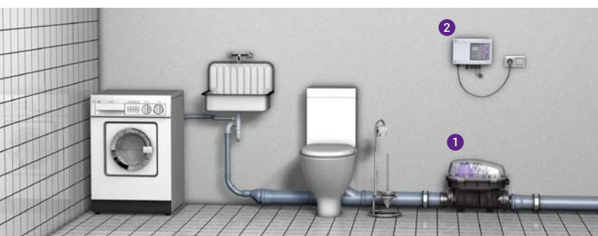
1 Backwater pumping station 2 Control unit
