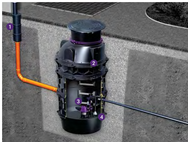
1 Gutter drain 2 Pumping station 3 Pump 4 Pressure sensor
