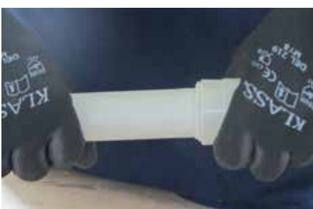
Finished socket fusion weld
