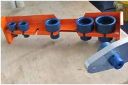
Scrape and chamfer the pipe
