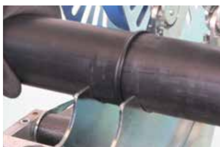
Finished butt fusion weld
